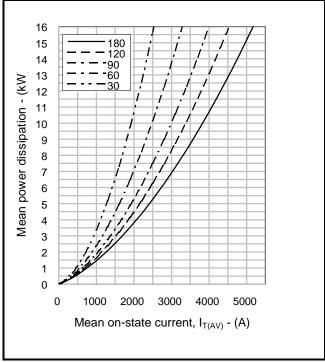
Fig.3 On-state power dissipation - sine wave
