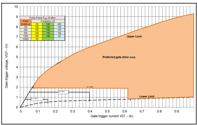
Fig14 Gate Characteristics
