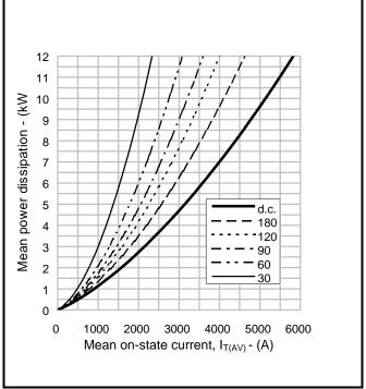
Fig.6 On-state power dissipation - rectangular wave
