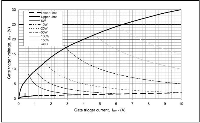
Fig. 15 Gate characteristics
