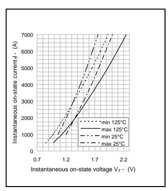
Fig.2 Maximum & minimum on-state characteristics
