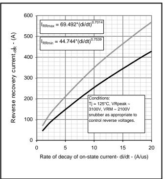
Fig.13 Reverse recovery current
